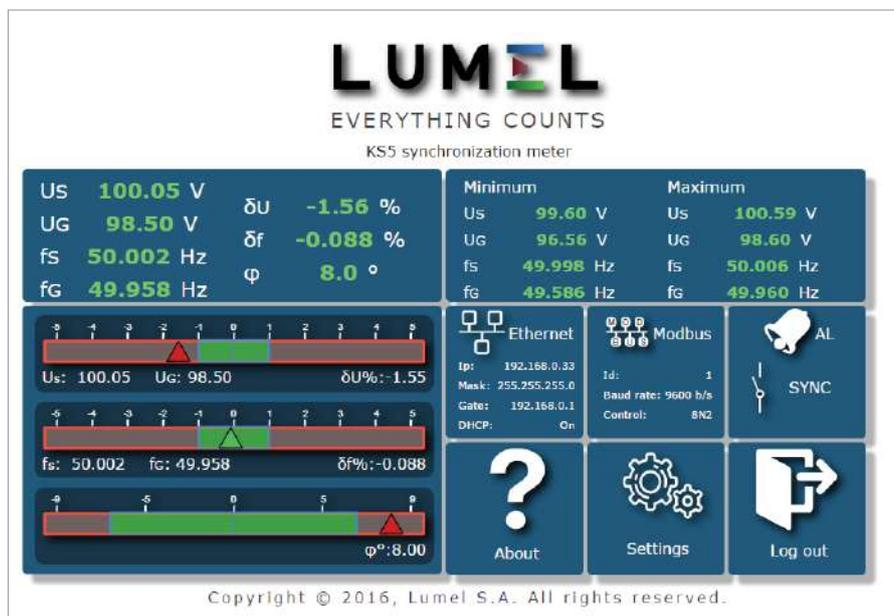
WEB server for remote reading of current measurement data
